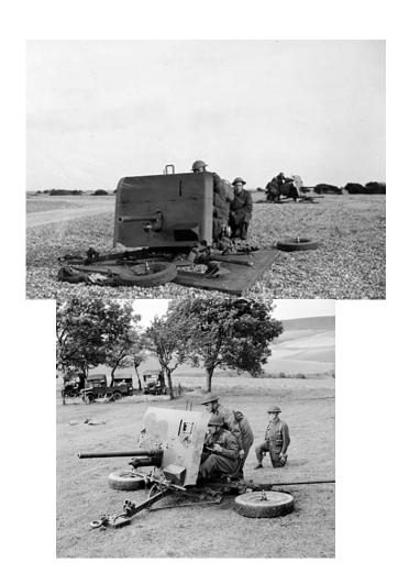
The 2 pdr was originally designed as a tank gun in 1934 to replace to obsolete 3 pdr gun but it was decided to mount the gun on an anti tank carriage when it was realised that Continental armies were deciding to provide 'light guns firing shell for anti-tank defence' also the adoption of the same weapon for both tank and anti-tank would be a great advantage
