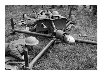
The Bombard was spigot gun - the projectile fitted on to a steel rod (or spigot) instead of into a barrel and was designed to be primarily an anti-tank weapon but could also be used in an anti-infantry role. It was intended to be a cheap anti-tank weapon and but also advantages over a standard anti-tank gun, it was much easier to conceal, required less manpower to operate and was much lighter.
